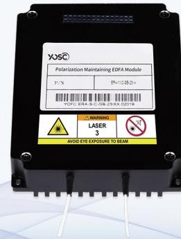
Polarization maintaining EDFA uses 980nm pump laser to provide energy. The polarization-maintaining passive devices have high output extinction ratio. The product can work in ACC/APC/AGC mode. The use of high-performance devices and accurate temperature control technology empowers the product good working characteristics in a wide temperature range, thus the product can be widely used in the field of optical fibre sensing.
