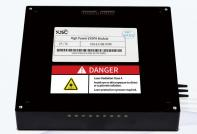
The high-power EYDFA adopts a two-stage amplifier structure, with the maximum output power up to 40dBm. It has been widely used in CATV system and FTTH. The product can work in ACC/APC/AGC mode and adopt high performance temperature control technology to empower the product good thermal performance in a wide temperature range.
