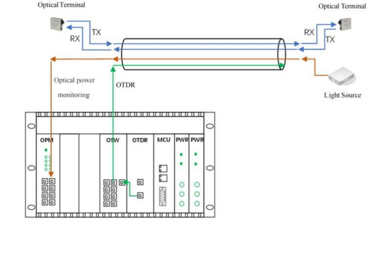
room; light source equipment installed in 7 branch server rooms permits real-time monitoring of the operator's main optical cables.
