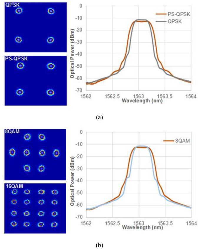
Fig.2. (a) Constellation diagrams and optical spectrum of QPSK and PS-QPSK (Constellation diagram of PS-QPSK just denotes a QPSK symbol which has been transmitted on the x-polarization) at 100G. (b) Constellation diagrams and optical spectrum of 8QAM and 16QAM at 200G.
