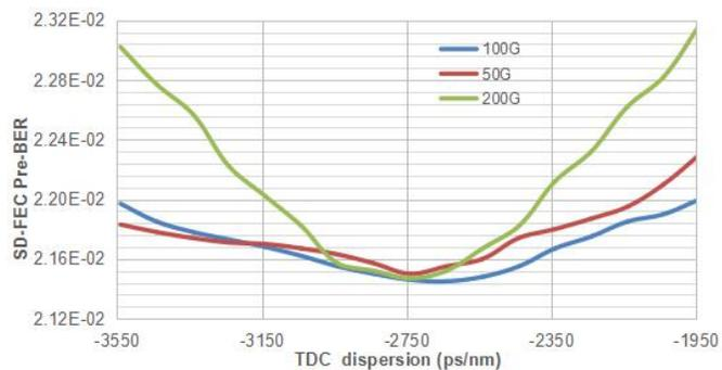
Fig. 13. Measured BER versus pre-compensation dispersion at 50G, 100G, and 200G.
