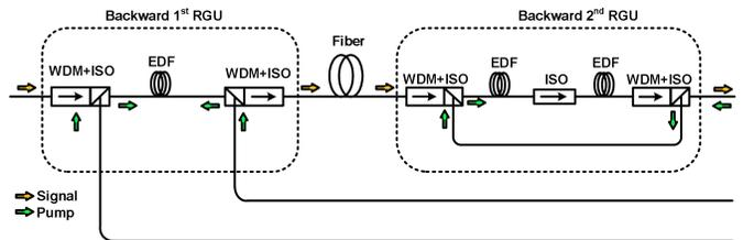
Fig.5. The structure of the backward cascaded RGUs
