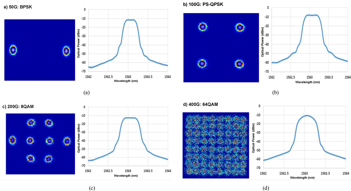
Fig.9. Constellation diagrams & spectrum of 50G(a), 100G(b), 200G(c), 400G(d) measured at the transmitter side.
