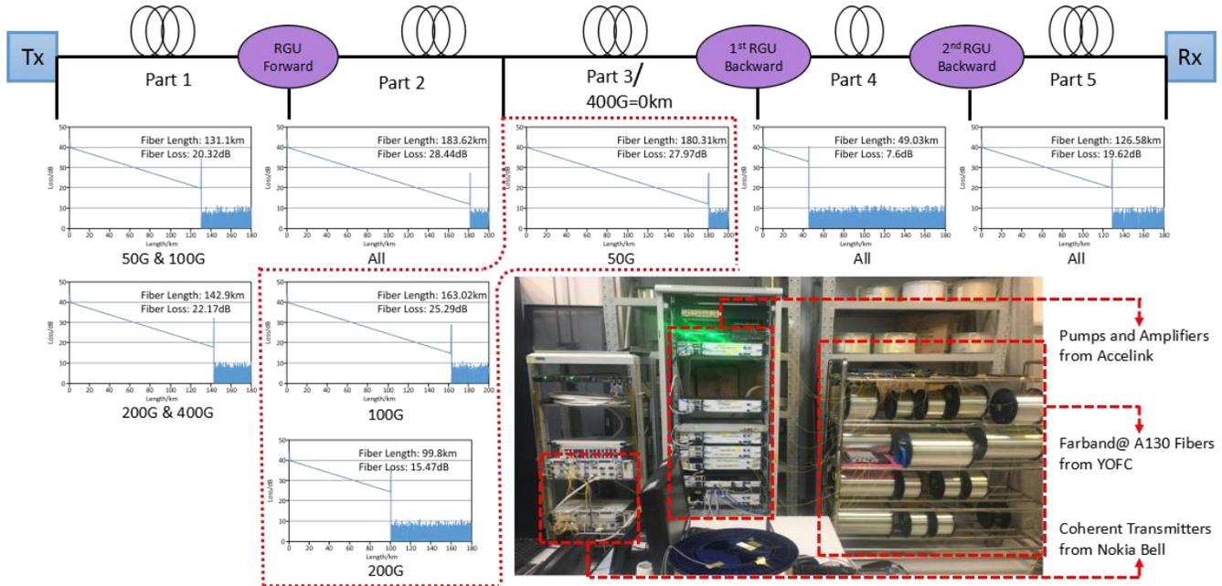
Fig. 8. OTDR analysis for transmission fiber and photograph of optical fibers and equipment.
