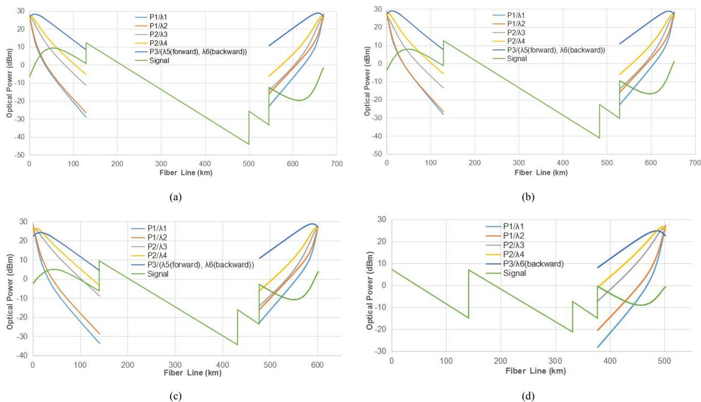
Fig.10. Simulated power distribution of signal and pumps in signal path for 50G(a), 100G(b), 200G(c), and 400G(d).
