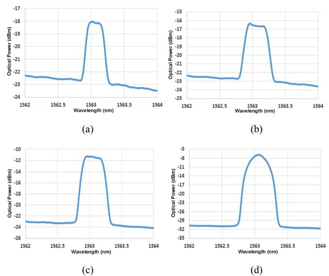
Fig. 14. 670.64km, 653.35km, 601.93km and 502.13km transmission spectrum measured at the coherent receiver for 50G(a), 100G(b), 200G(c) and 400G(d).
