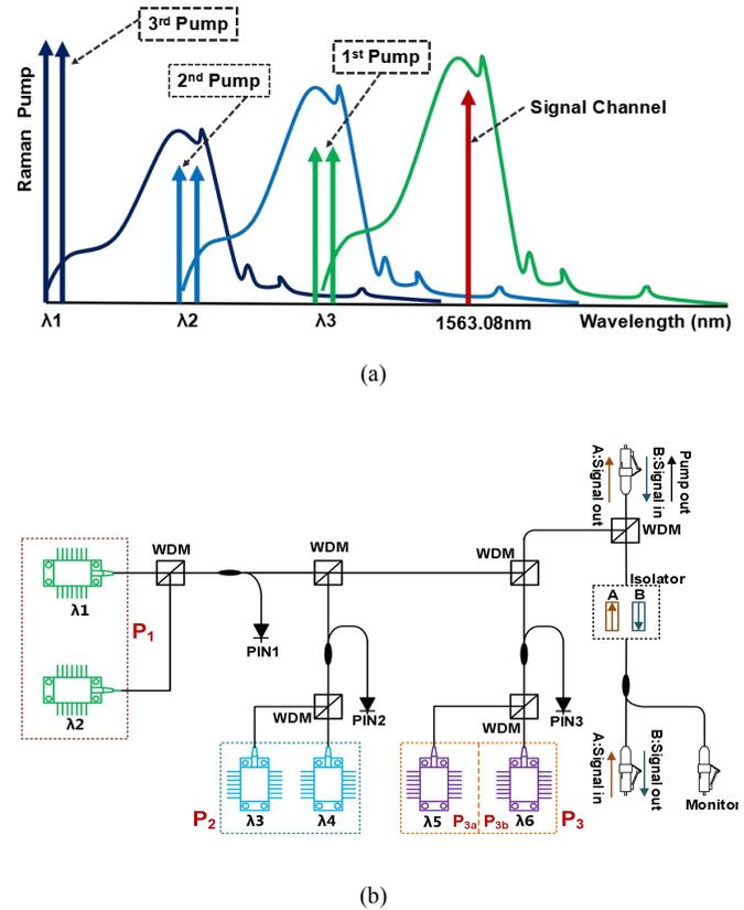
Fig.4. (a) High-order Raman gain spectrum with different pump laser wavelengths. (b) Structure of HRP.
