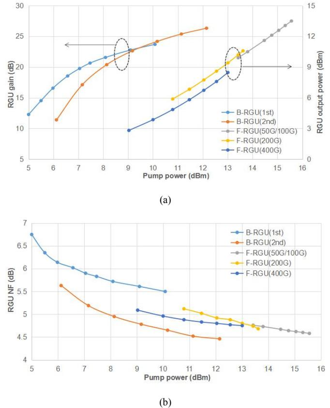
Fig.7. (a) Output optical power of forward RGU and gain of backward RGU versus pump power. (b) Noise figure of RGU versus pump power.
