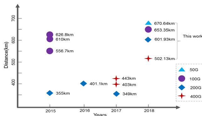
Fig. 1. History of record distance of unrepeated transmission with several generations of channel bit rate.
