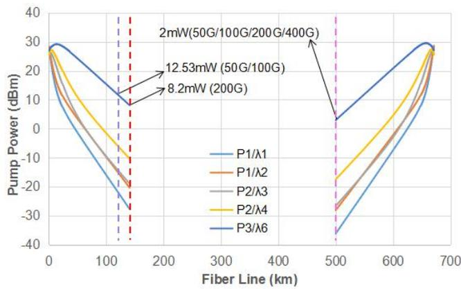
Fig. 11. Simulated power distribution of pumps in pump path.
