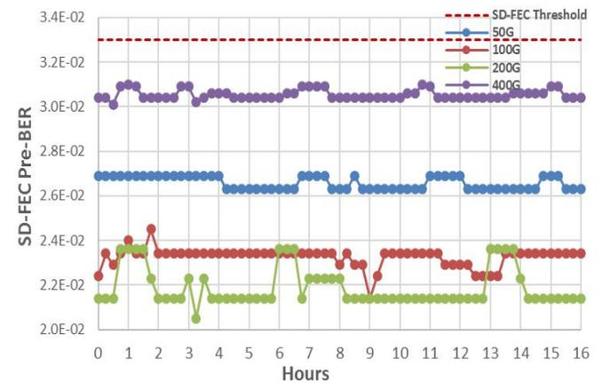
Fig. 15. Stability measurement over 16-hour at 50G, 100G, 200G and 400G.
