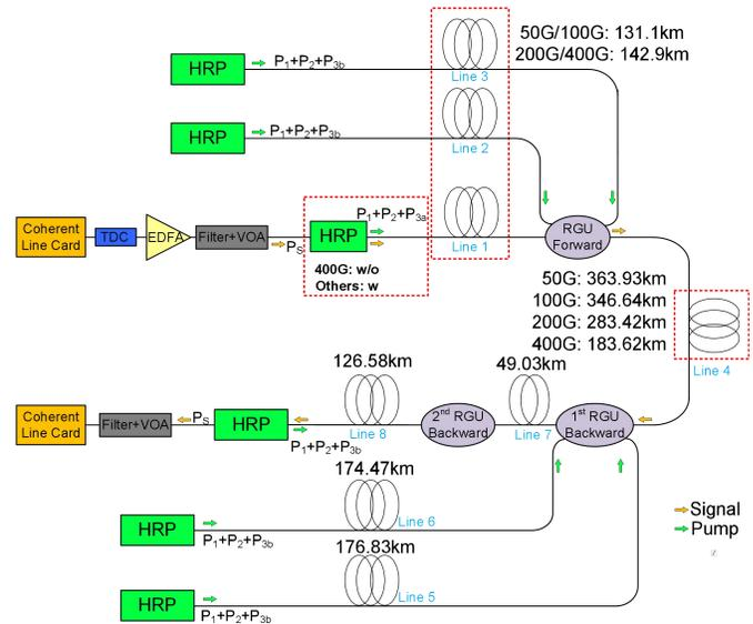
Fig.6. Experimental setup for single 50G/100G/200G/400G channel unrepeated transmission. Insert (dashed box) shows the different configuration used for 50G/100G/200G/400G transmission.
