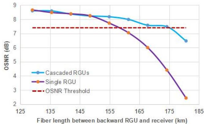
Fig. 12. OSNR comparison between cascaded RGUs and single RGU.
