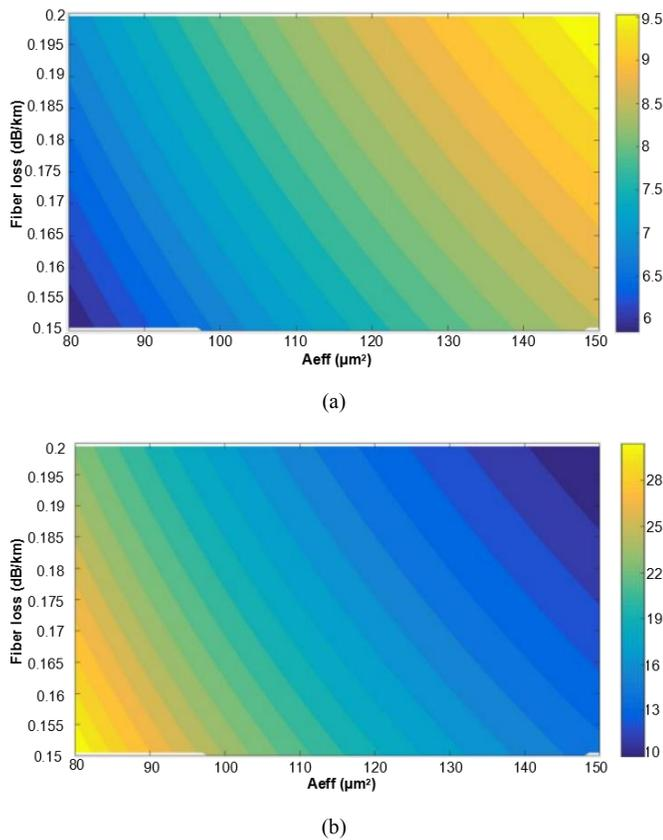
Fig. 3. (a) Optimum launched signal power into fiber, and (b) Raman gain with total pump power of 1 W as a function of fiber loss coefficient and effective area based on 400 Gbit/s system.
