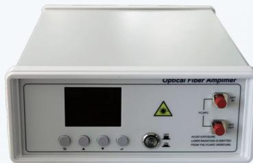
Benchtop Polarization-maintaining EDFA is specially designed for fibre optic sensing, communication system, laboratory testing, etc.. Low noise 980 pump laser and polarization-maintaining passive components are adopted to ensure relatively high extinction ratio. it operates in ACC or APC mode. Based on fine temperature control technology inside and satble components, it provides excellent temperature characteristics even under harsh working environment.
