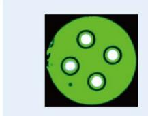
4-cores single-mode fibre
