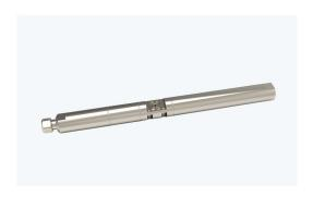
It is equipped with a fusion box and adopts a metal to metal sealing connection design, which can achieve the connection and sealing between the fibre optic pressure sensor and the 1/4 armored optical cable. It is fully suitable for the long-term monitoring of underground annulus, pipeline or port pressure.
